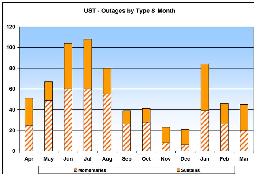
The metric used to track the total disturbances rate is TSAIFI (the total number of disturbances per circuit-year). The FY2008 result for this metric was 1.17, indicating there was, on average, slightly more than one disturbance per circuit over the year. The actual break-down of disturbances for the year was 374 momentaries and 262 sustained.
